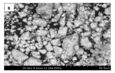
Fig. 4: SEM images of Silver Nanoparticles synthesized from *B. flexus and B. pseudomycoides*
